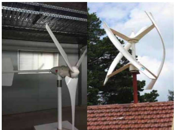
Figure 3: (left) the HAWT at the NHP Sustainability Centre (right) a VAWT courtesy of True Solar Time.
