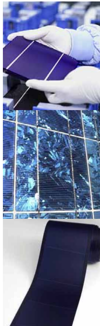
Figure 2: (top - bottom) Mono-crystalline, Poly-crystalline and thin film solar cells (3)
