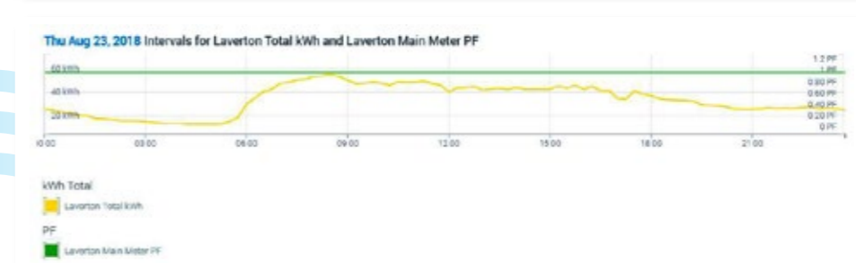
The above images showcase the before and after installation of the SVG unit. Before turning on the SVG unit, the power factor (green line) is shown to vary down to 0.8 around 4pm on August 22, 2018, the moment the SVG unit is switched on the Power Factor improves instantly and remains at target power factor under all load conditions. (This is all data captured via InfoSyte – this has not been manipulated).
